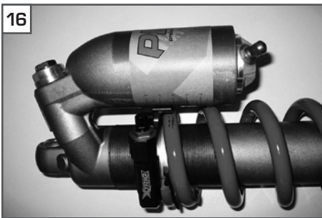
Mount the sticker with the scale on the compensating tank to make it easier to adjust the preload.
