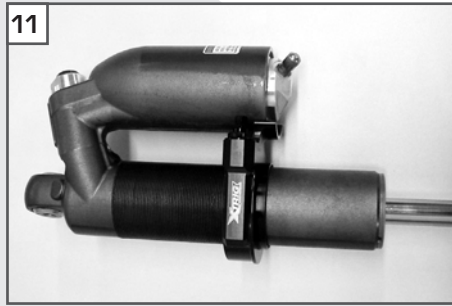
Turn to at least half of the Preload Adjuster mount and check whether the position is correct.
