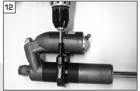
When you pass the middle of the mount you can turn the Preload Adjuster with a cordless screwdriver instead of the T-wrench for faster mounting.
