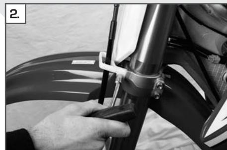
Remove the brake line guide.
