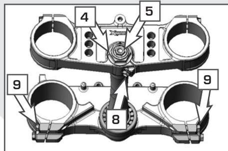
To change the offset, jack up the motorcycle under the frame, lifting the front wheel off the ground. Remove the front fender. Loosen the 5 clamp screws ( 8 ) and ( 9 ) and remove the two screws ( 7 ). Push the lower triple clamp down approx. 22 mm, making sure the fork is not compressed in this state.
