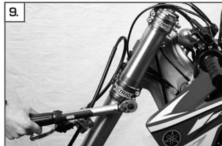
Tighten the clamp screws ( 9 ) on the lower triple clamp to 15 Nm. Mount the front fender and brake line guide.
