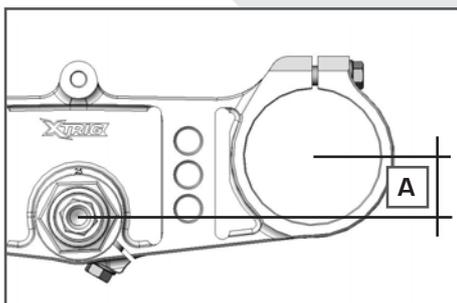
The Xtrig triple clamp can be used to adjust the fork offset [ A ] (center of the fork legs – center of the steering head bearing) to adapt the handling to the racecourse.
