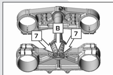
Turn the adjusting nut ( 4 ) on the steering stem 180° in a clockwise direction using a suitable wrench (A/F 27). Make sure you do not loosen the counter screw ( 5 ). Remove the collar screw from the hole ( B ) (if used) and push the lower triple clamp all the way up again. Screw in and tighten the two screws ( 7 ). Tighten the 5 clamp screws ( 8 ) and ( 9 ) and mount the fender. Check the steering head bearing clearance and readjust if necessary.
