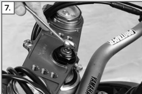
Screw the counter screw ( 5 ) in the adjusting nut ( 4 ) and tighten to 10 Nm.
