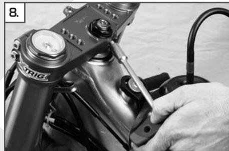
Tighten the collar screw ( 8 ) to clamp the shaft tube to 20 Nm.
