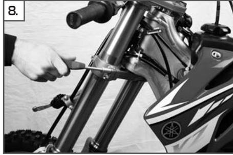
8. Loosen the triple clamp clampings.
