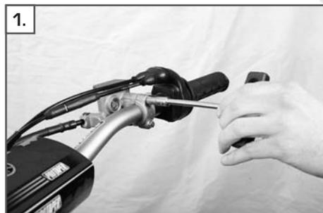
Remove the brake pump.
