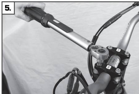
5. Screw in the M8x45 screws (11) evenly and tighten with 20 Nm. Make sure that the clamping gap between the shells (7) + (10) is the same (See picture right / wrong)
