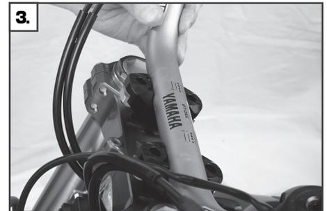
3. Mount the handlebar and move it into the desired position.
