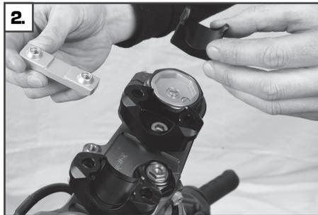
2. Insert the clamping bar (6) into the base support (2) (cone facing up) and snap the lower handlebar cup (7) into the clamping bar (6).
