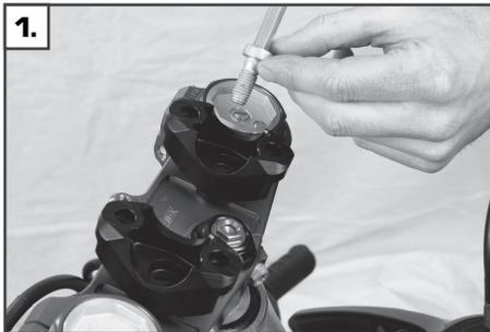
1. Screw the base carrier (2) with the pre-assembled rubber cone (3) onto the fork bridge (M10 x 25) (4) and screw tight with 40Nm. If necessary, add handlebar risers (1), but use the M10 x 35 screws (5) **NOTE: Ensure that the offset direction is the same.**
