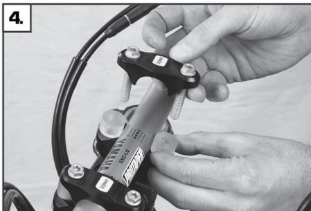
4. Put on the upper handlebar cups (10) with the pre-assembled intermediate rubber (9), screws M8x45 (11) and elastomers (8).
